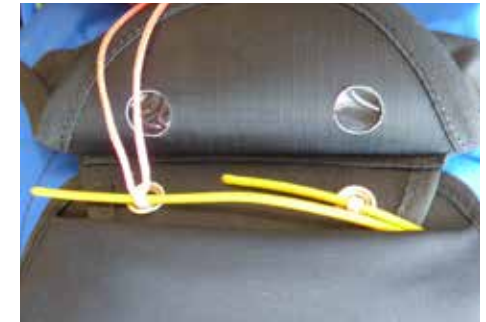
Push the Loop through the upper grommet flap grommet and push the yellow cable through it ( loop ).
